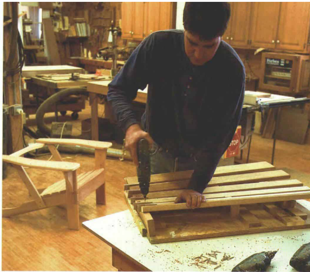
Building the back. A jig holds the bottom and upper back stretchers while the author screws on the back splats. He uses spacer blocks at the bottom and middle of the splats.
