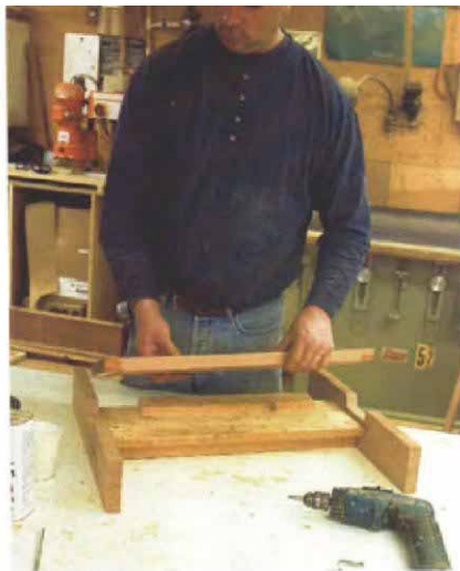
Front stretcher is let into the front legs. Both long edges of the stretcher are ripped with the saw tilted 20°—the same bevel at which the rear legs meet the front legs. A simple jig (right) holds the front legs at the proper spacing.
