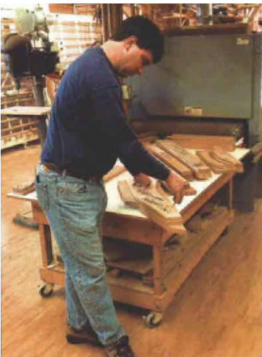
Front stretcher is let into the front legs. Both long edges of the stretcher are ripped with the saw tilted 20°—the same bevel at which the rear legs meet the front legs. A simple jig (right) holds the front legs at the proper spacing.
